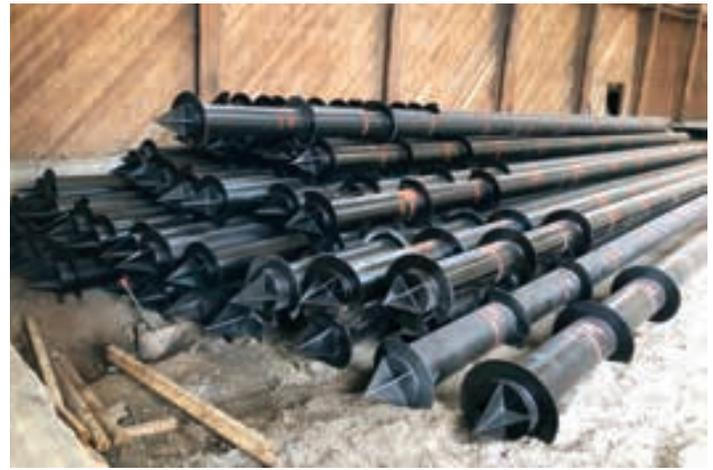
**PC-CIDH steel casings with fabricated pile points**
